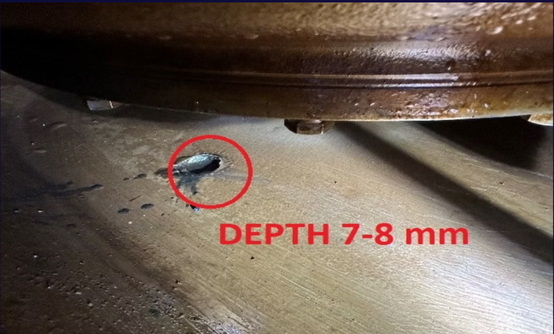
Deep cavitation erosion (7-8 mm)
