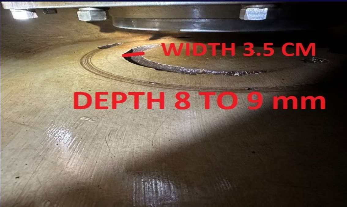
Severe cavitation erosion (3.5 cm wide, 8-9 mm deep)
